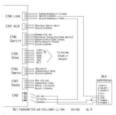
Wire the Super Scan to the ACTUATE input instead of the AUX input and put the normally open side of the lock relay in series with it. (I am assuming since the door can be used manually, there's no lock. This won't work without an extra relay and more wiring hassle if the lock relay contacts are already in use to operate a lock).
