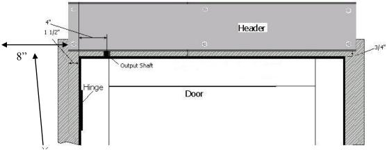
**NOTE:** If door is an In-Swing, allow 8" minimum between header and opposing wall to allow clearance for the Pull Arm.
